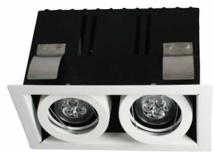
MR16有邊框崁燈(2燈) 開孔147*79外徑68高度94MM
